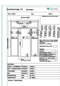
This form is for a block frame part 3 (with side panel and glass). It includes sections for door type (e.g., Schiebetür), dimensions (Width: 1000 mm, Height: 2000 mm), door leaf (Standard), door handle (Standard), and accessories (Standard).
